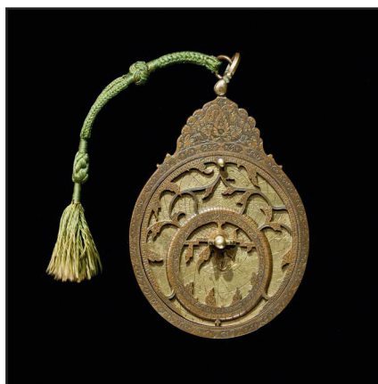
This bronze astrolabe, made in Persia circa 1730-1775 and on display at the NY exhibition (left), has several inset plates for use by travellers at different latitudes.
